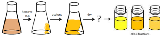
Figure 3: The isolation and purification of Flexirubins. The steps from acetone extract to HPLC fractions of different flexirubins as represented by "?" are the focus of this project.
